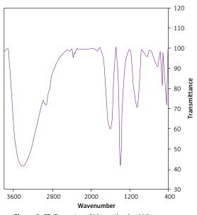
Figure 2. FT-IR spectra of biosynthesized Ni nanoparticles
